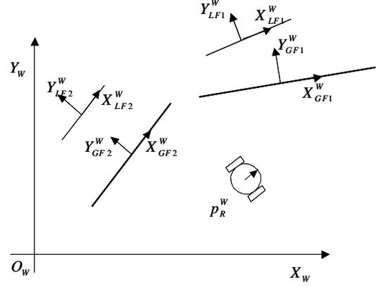
Figure 3: Relations of the robot and line segments
