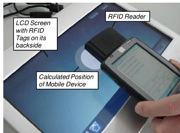
Figure 2. Prototype system in use
