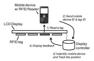
Figure 1. System configuration.
