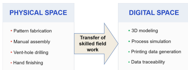
Fig. 1. Conceptual definition of digital casting as the transfer of skilled field operations from physical space to digital space.
